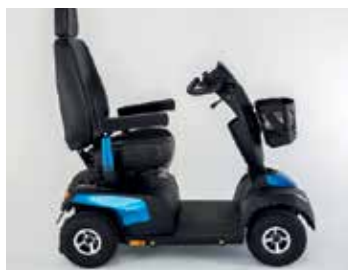
Seat suspension module offers additional comfort by adding an optional seat suspension.
