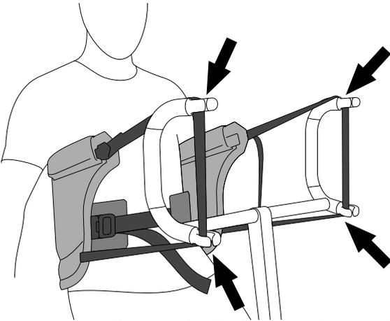
Fasten the sling to the lifting arm by guiding the strap into all 4 hooks.
