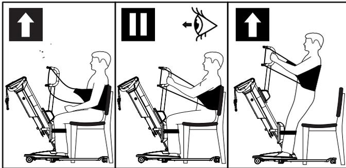
1. Check that the sling is correctly fitted around the user and that the strap loops are correctly fitted to the suspension hooks.
