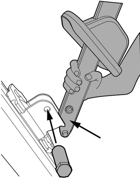
Place the cover onto the lifting arm. Place lifting arm in trolley, and insert the bolt.
