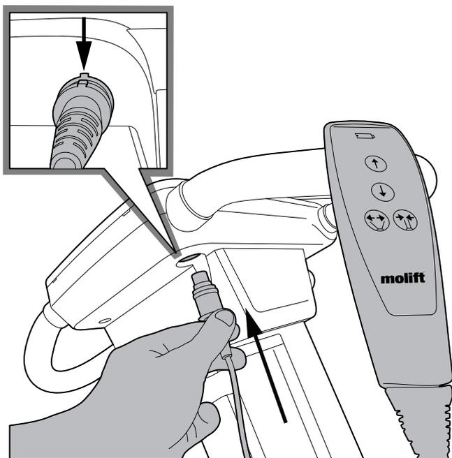
Connect the hand control to the control panel.
