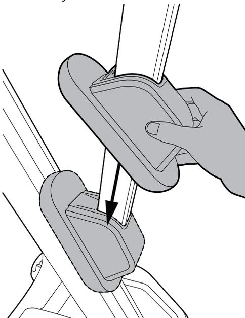
Fit the cover onto the trolley
