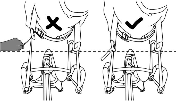
Pull the loose strap to adjust the length of the straps. Make sure both sides have equal length.
