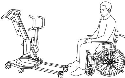
Move the Quick Raiser 205 in front of the user. Place the feet on the footplate. If necessary - help the user to place the feet correctly. Lock the wheels on the lifter before lifting the user. The optimal angle of the users joints before lifting is 90 degrees.
