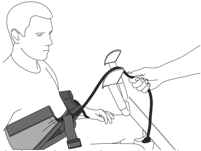
On the 2-point suspension arm the ropes is attached to the lifting arm by pulling them firmly from above and into the rope locks.
