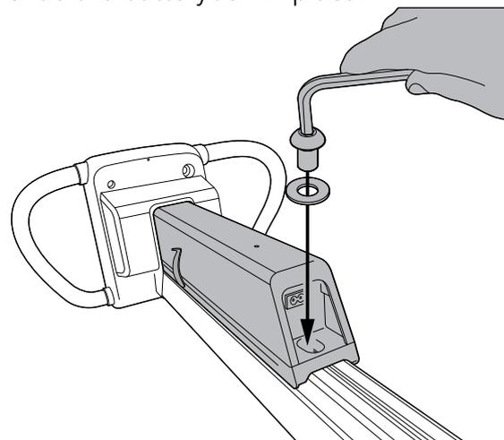
Use the allen key and tighten screw clockwise. NB! make sure to use the washer.
