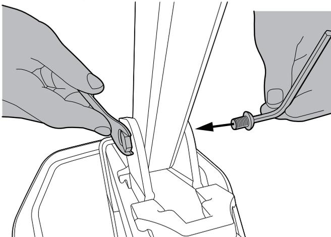
Insert the bolt and tighten the screw using the 17mm spanner and an 6mm allen key. Make sure the lifting arm is properly fastened to the trolley on the column.
