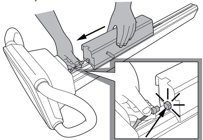
Place the column on a horizontal surface. Make sure the emergency stop is pushed in. Connect wire from control panel to battery box. Slide the batterybox in place.
