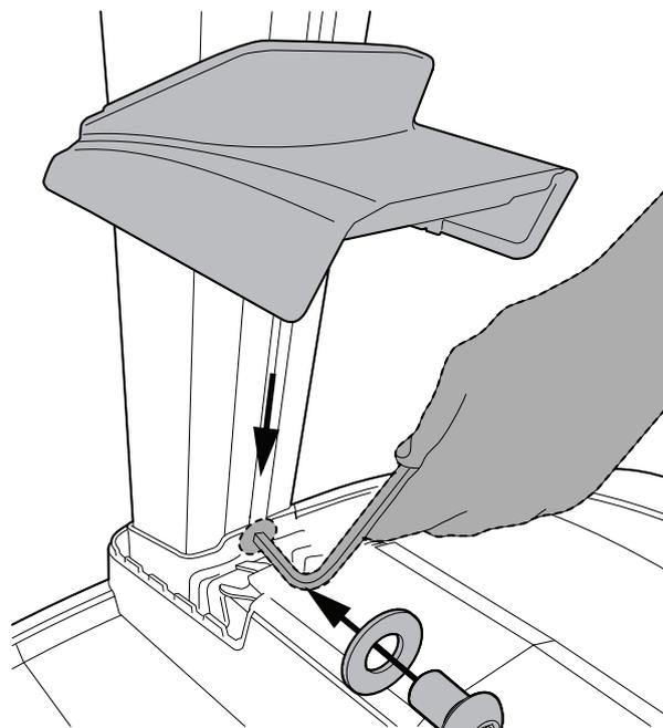
Mount the screw with washer on column. Slide the screw down to chassis, and tighten the screw.
