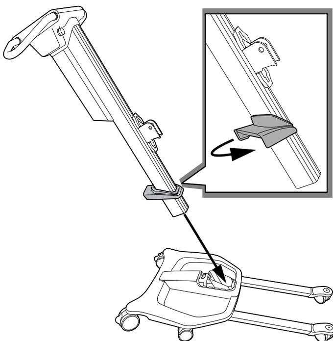
Place the cover on to the lifting column. Twist the cover sideways to make it stay on column. Insert the lifting column into the chassis.
