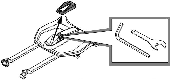
Locate assembly tools (5mm allen key, and 17mm spanner)
