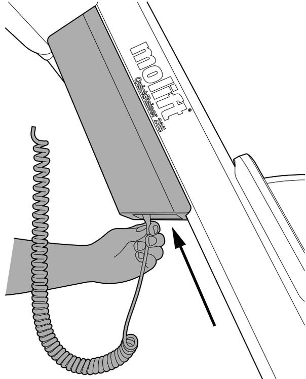
Connect the mains cable to the bottom of the battery box.
