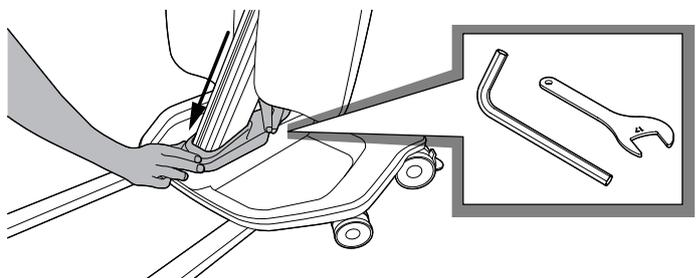
Fit the cover on to the chassis. Remember to put the tools back in place.
