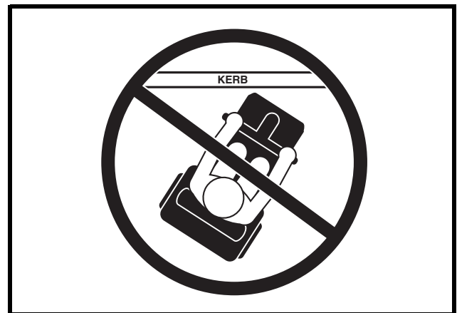
Figure 3A. Incorrect Kerb Approach
