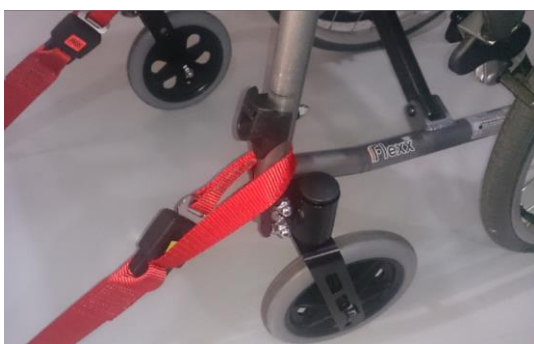
Fitting the Front Restraint
